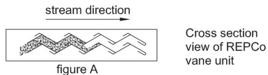
Separation (and/or recovery) of the liquid occurs continuously and consistently under full process operating pressure and remains unaffected by varying flows and conditions that are induced by reciprocation, pulsation, or centrifuge equipment upstream and/or large turndowns that are often experienced by multi gas turbine power plant.
